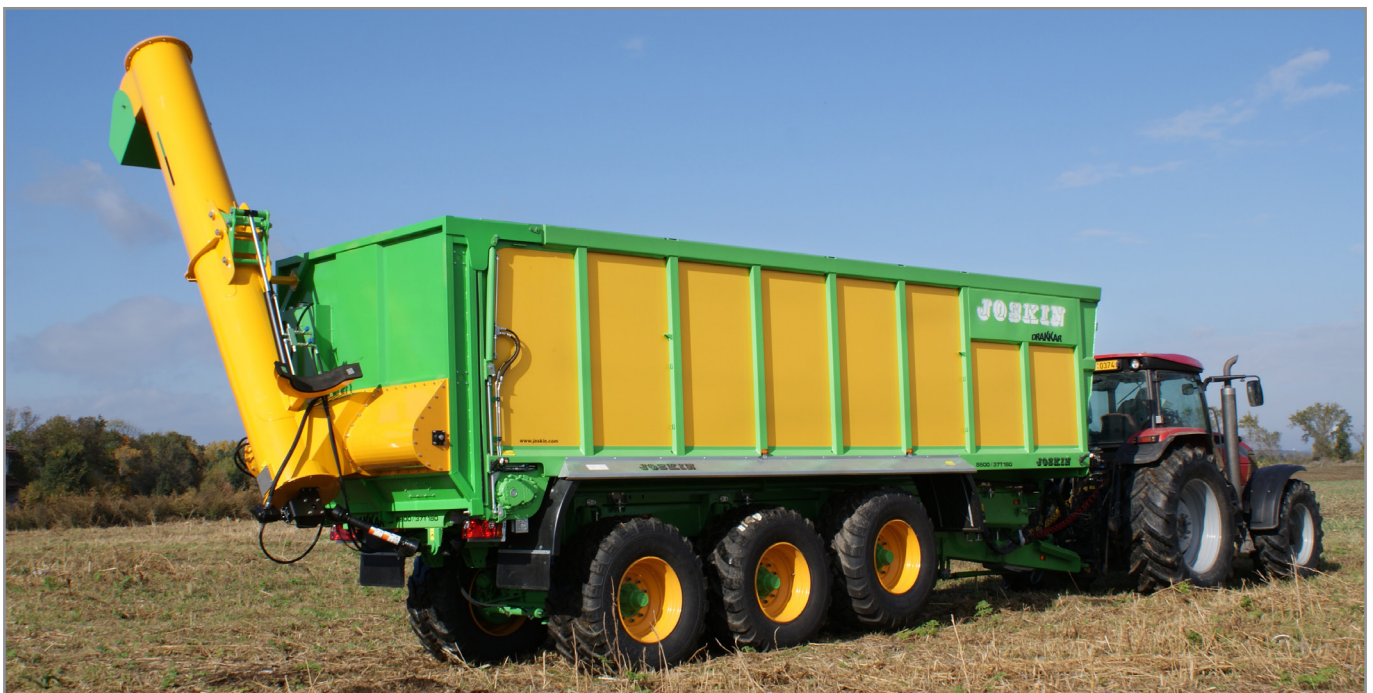
DRAKKAR with transfer auger and dynamic weighing system allowing to comply with the regulations in force when unloading in a semitrailer.
